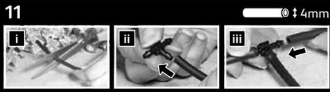
Occasional slight leakage can occur from the Supply Tube / Micro Tube connection point. This usually seals over time, but ensure the fitting is correctly inserted at a 90° angle.
