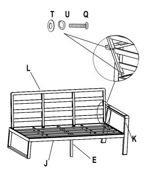
**STEP 7:** Attach Back Rest 3 (L) to the Armrest 2 (K) using the M6x55 Bolt (Q), Lock washer (U) and Washer (T)
