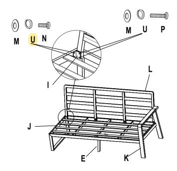
**STEP 8:** Attach the Connector Bracket (W) to Back Rest 3 (L) using the M6x45 Bolt (P), Lock washer(U) and Washer (M). Attach the Connector Bracket (W) to Seat board 2 (J) using the M6x20 Bolt (N) , Lock washer(U) and Washer (M)
