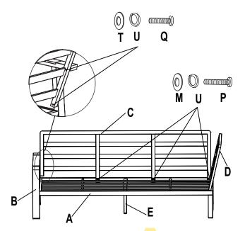
**STEP 3:** Attach Back Rest 1 (C) to Seat board 1 (A) using the M6x45 Bolt (P), Lock washer (U) and Washer (M). Attach Back board 1 (C) to the Armrest 1 (B) using the M6x55 Bolt (Q), Lock washer (U) and Washer (T)
