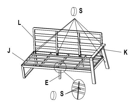
**STEP 9:** Tighten all the bolts on the leftside sofa and cover with the Plastic bolt cap (S). Turn the sofa over.
