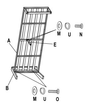
**STEP 1:** Attach Armrest 1 (B) to the Seat Frame 1 (A) using the M6x35 Bolt (O), Lock washer (U) and Washer (M).
