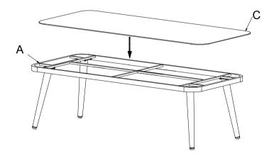
**STEP2:** Turn the table over and place the Glass(C) onto the Table top(A)
