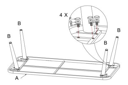
**STEP1:** Attach Table leg (B) to the Table top (A) using M6x15 Bolt (D) and Washer (E). Tighten all the bolts and finish with the Plastic bolt cap (F)
