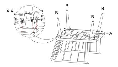
**STEP1:** Attach Legs (B) to the Seat Frame (A) using M6x15 Bolt (E) and Washer (F). Tighten all the bolts and finish with the Plastic bolt cap (G)
