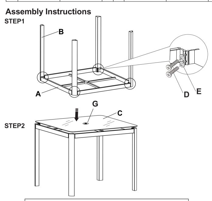
PLEASE ENSURE ALL FIXINGS ARE LEFT LOOSE DURING ASSEMBLY BUT ARE SECURELY TIGHTENED UPON COMPLETION.
